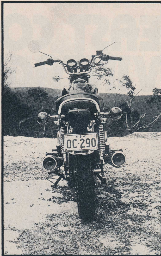
All that rubber on the road looks impressive but in the wet the tyres are ineffective. Rear is a Yokohama 4.10-18, front a Yokohama 3.60-19. The bike is slim, the widest part being the bars. Side stand is difficult to put down despite the large horn, but it tucks neatly up under the silencers and doesn't scrape.
