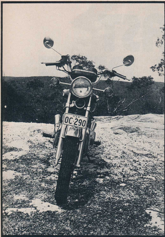
All that rubber on the road looks impressive but in the wet the tyres are ineffective. Rear is a Yokohama 4.10-18, front a Yokohama 3.60-19. The bike is slim, the widest part being the bars. Side stand is difficult to put down despite the large horn, but it tucks neatly up under the silencers and doesn't scrape.
