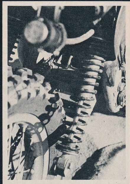
Swingfork is double braced behind pivot point for maximum rigidity. Entire frame is very rigid.
