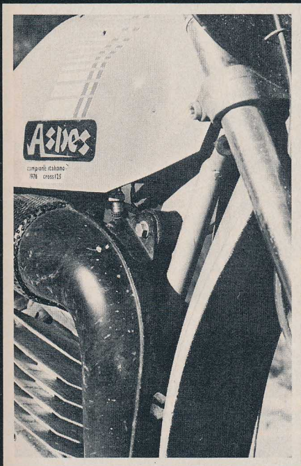
Front right-hand petrol tap is very hard to get at after engine has been running and chamber is hot. Note rubber mounting of exhaust to frame.
