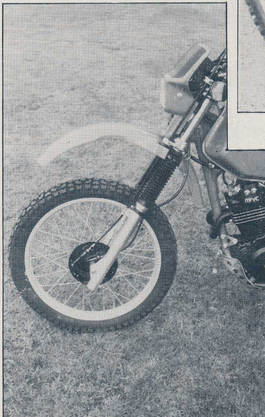
Single leader did its job adequately. Front guard is plenty long out forwards but a bit short on at lower for engine protection
