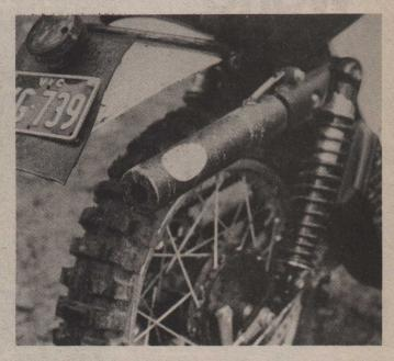
IMITATION RIM PROTECTOR!!! A good 4.25 x 18 6 ply Bridgestone enduro tyre would naturally make a lot of difference but the problem would still be there as a basic characteristic of the machine demanding it to be ridder accordingly. It's just that there is so much raw torque available every little bit helps.
