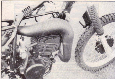
Engine runs reasonably quiet due to rubber blocks in fins
