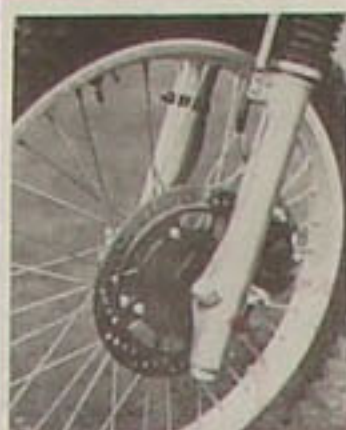
The disc brake on both models - superb and unaffected by the conditions.
