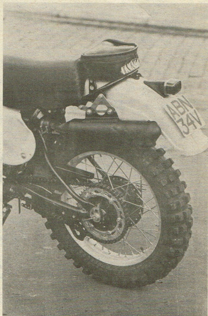
The business like back end of the IT has a QD wheel, handy tool bag and a noisy silencer.
