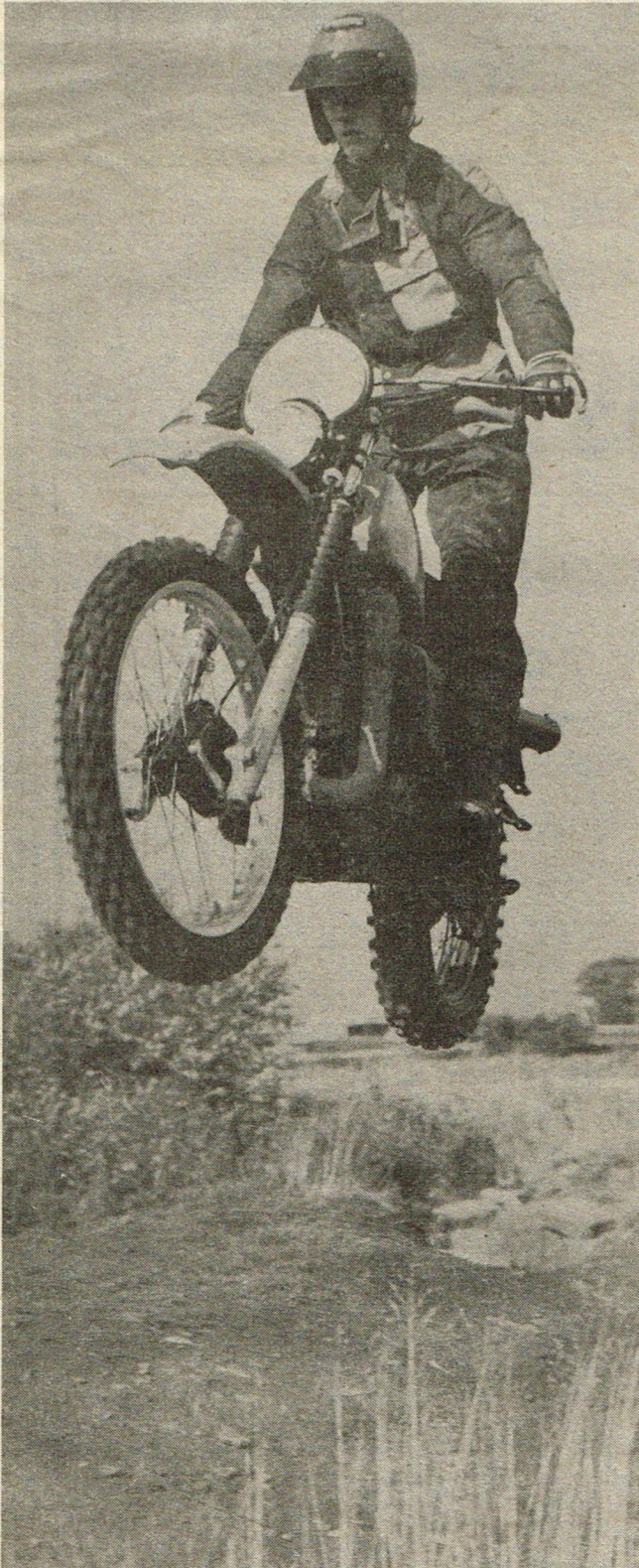
A landing from this height will usually soak up all the available travel. More travel would also mean more seat height.
