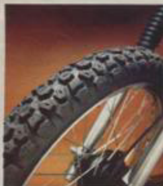
Dunlop K150 rubber is good on the road, less so off it
