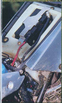
Left: Battery lives under the seat - exposed connectors not so good. Centre: Toolkit comprehensive but bulky. Right: Filler at rear
