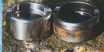
New stainless spacer on left, original mild steel on right...
