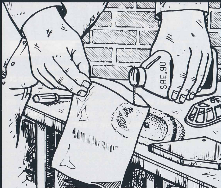
One way of applying oil to your air filter is to pour the oil into a plastic bag and drop the filter in afterwards, working the oil well into it...
