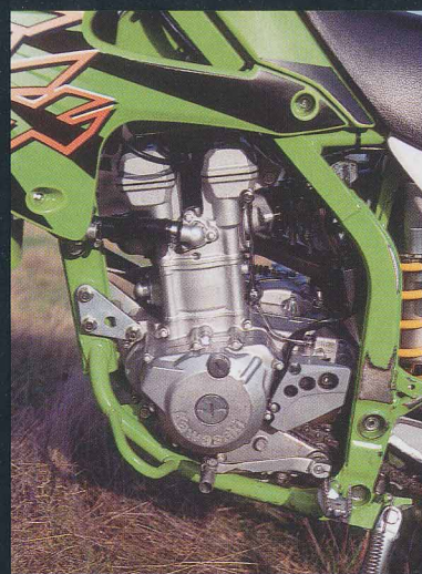
DOHC motor is a real gem. It revs to 11000rpm and has no flat-spots anywhere in the rev range. Sadly the gearbox can't match the engine's qualities - there's far too many neutrals waiting for the unwary. Headlight only lasted 45 minutes in Pavey's hands...
