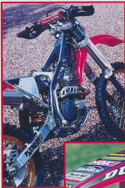
Right: Hand-made pipe adds to the Monnier's sound but not its mass
