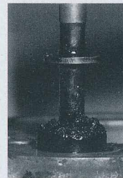
Photo A shows a Kawasaki KR1S 250cc 2 stroke power valve before using PowerPill treated fuel. The mix partially burned fuel, oil and carbon flakes coat the stems heavily
