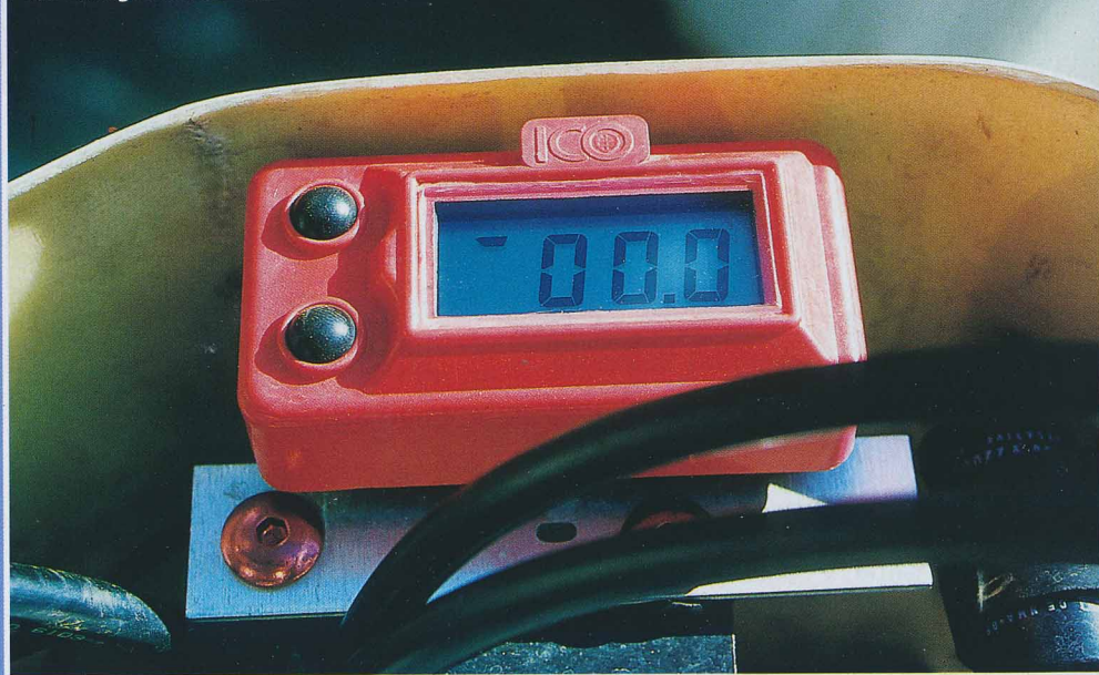
An electronic ICO meter replaced the damaged Honda dials
