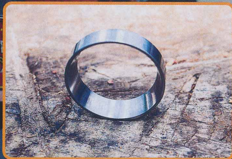
LEFT: The grooves in this cone show why a worn bearing gives notchy steering
