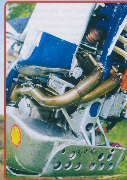
Look how close the fuel tank is to the header pipe.
