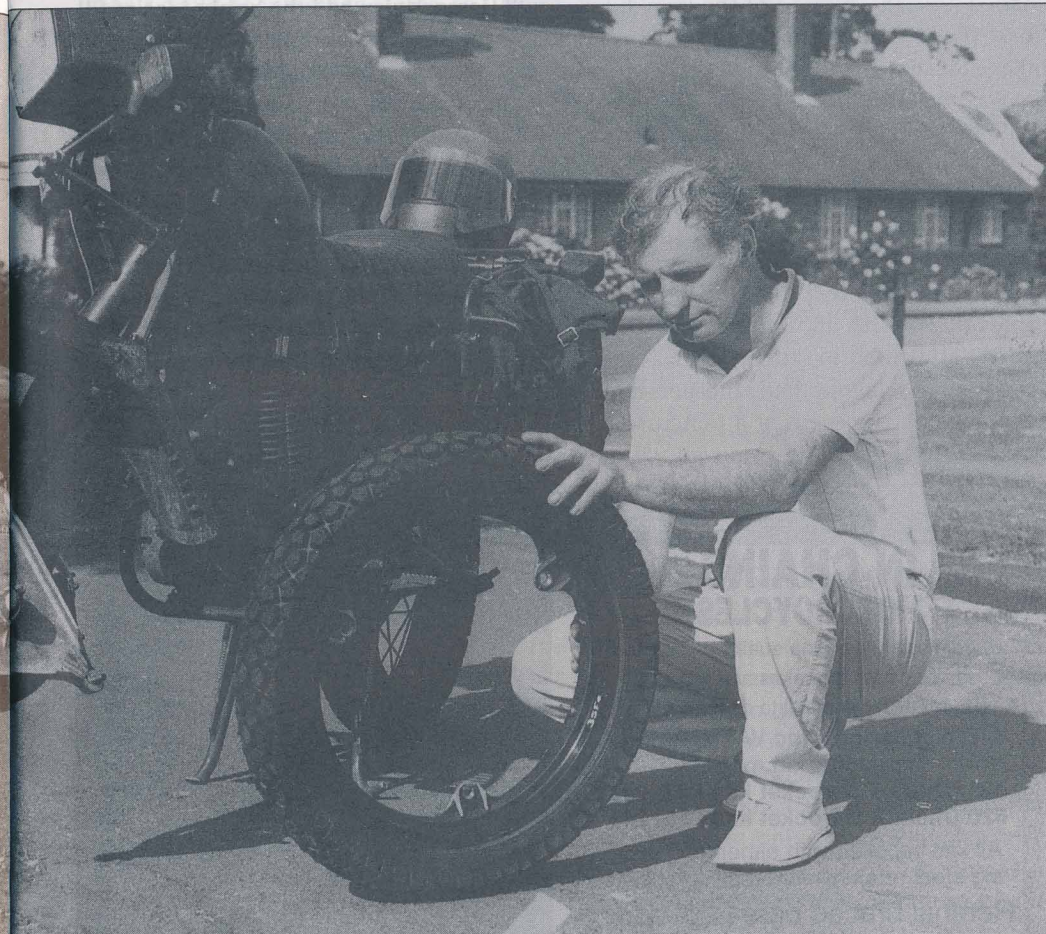
It's 1987 and Norman Hossack demonstrates the simplicity with which a tyre (and wheel) can be removed from the army bike
