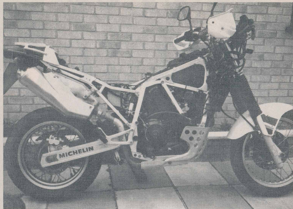
Stripped bare, the Elefant displays its compact packaging. Extended sump shield gives extra protection to exhaust and rear linkage
