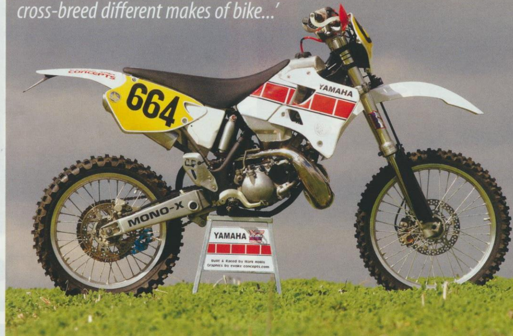
Suspension and brakes are lifted off a YZ426. Period YZ200 stickers finish the job...
