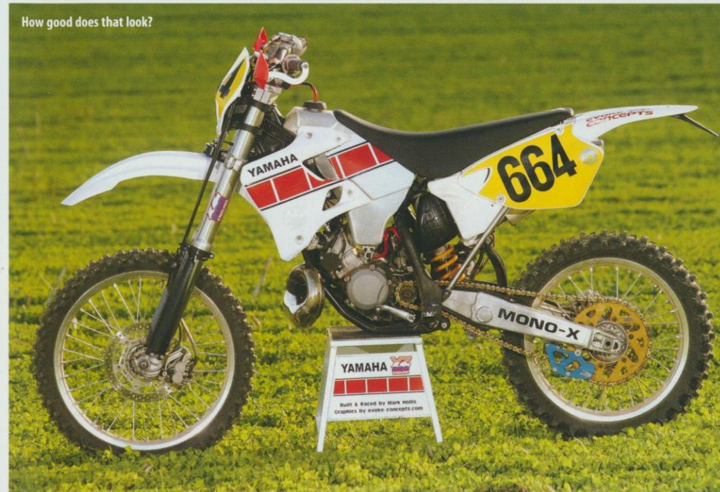
Mark changed the angle of the bike's pipe to help it clear the kick-start...
