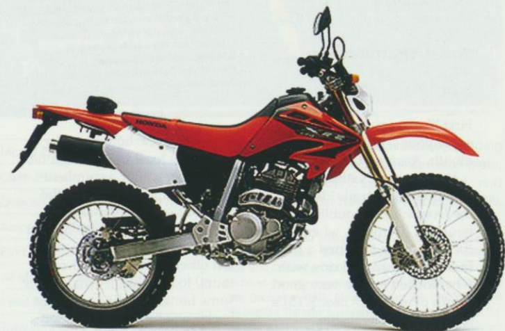
Reader David Nicholas is looking for an imported Japanese-spec Honda XR250R to use as a commuter bike. This machine differs from the UK bike by dint of its electric-start motor, upside-down forks, CRF styling and road-legal kit. Not quite as powerful either...
