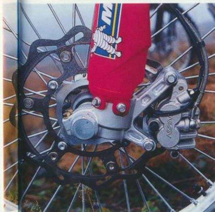
Above: Elegant simplicity and attention to detail gives the Beta its good looks. Below: Opting for a Nissin/Braking disc set-up provides superior feel. Right: All wrapped up: KTM 450 power-plant looks right at home in the Beta
