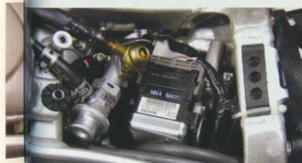
Above: Fuel injection gubbins lives under the seat. Right: 4RT motor is based on the CRF lump. Below: New bike is a far cry from Montesa's 1967 model
