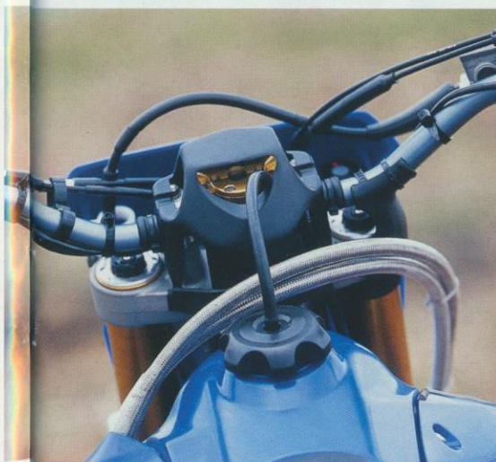
Fluid drive goes up and over the tank, but never seems to get in the way. Steering damper is essential on the AWD bike because of the effect of engine braking from the front end! Right: Fluid pump bolts onto the outside of the WR's output shaft, but isn't obtrusive...
