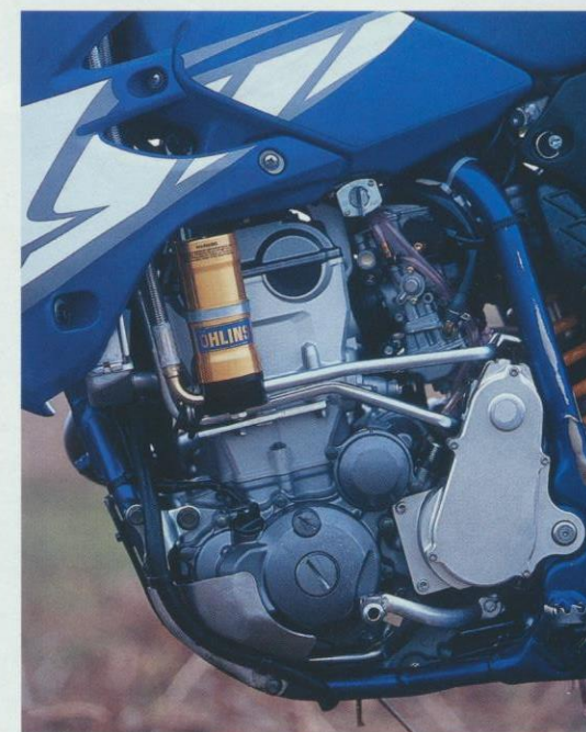
Fluid drive goes up and over the tank, but never seems to get in the way. Steering damper is essential on the AWD bike because of the effect of engine braking from the front end! Right: Fluid pump bolts onto the outside of the WR's output shaft, but isn't obtrusive...
