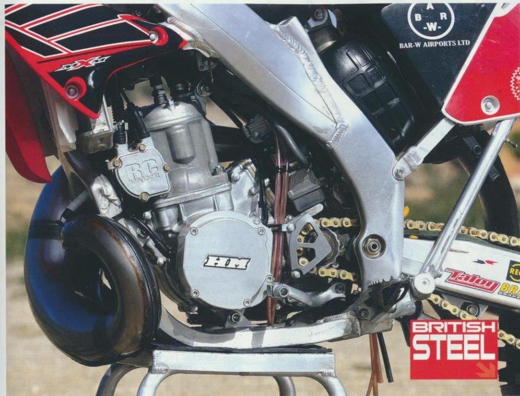
Above left: The Honda's triple clamps come courtesy of Pulse Racing, the bar mounts offering Eddy a range of positions. And don't those MXM graphics look good...! Above: The CR motor has been tuned to meet Paul's requirements, with a 2C pipe and an HM lighting coil... Below and below right: Braking discs and Talon sprockets are employed. Front axle puller is standard WEC kit...
