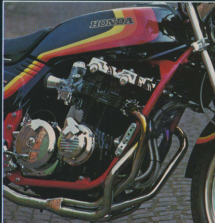
The frame was beadblasted before two coats of primer and two of red were applied. Engine is finished in Sperex gloss black
