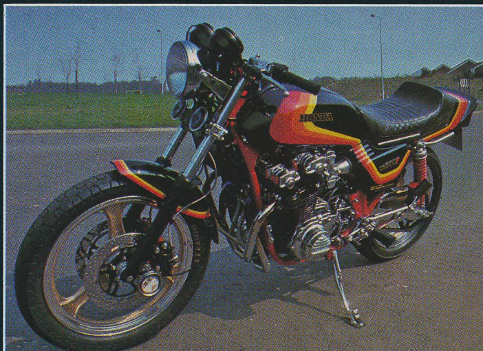
Front and rear guards are cut down. Alloy footrest plates are sculpted out with chromed outside faces
