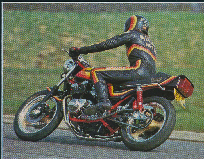
The frame was beadblasted before two coats of primer and two of red were applied. Engine is finished in Sperex gloss black
