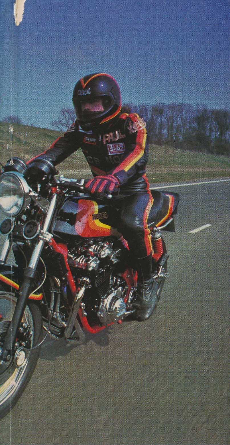
The frame was beadblasted before two coats of primer and two of red were applied. Engine is finished in Sperex gloss black
