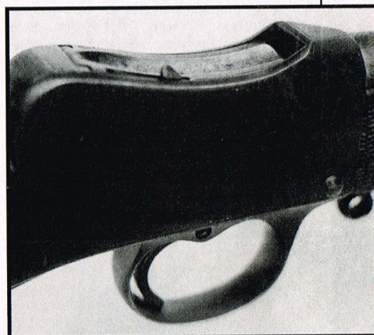
Cocking indicator of Greener's Martini seen protruding when striker at full cock.
