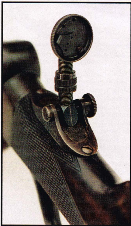
Greener patented features of both ladder and aperture sight, presumably the traverse adjustment for the windage. Sight was very finely made.
