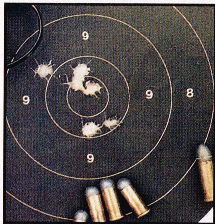
Groups with Krank's 'Fine' black powder and .375 swaged Hornady ball at 50 yards were excellent. Note original round of .380 long to right for comparison.
