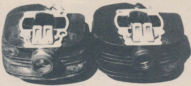
More finning round the block for better heat stability, also round the head.
