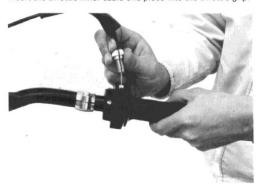
Turn the throttle grip clockwise fully, and set the throttle inner cable end piece to the slot in throttle grip body.
