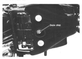
Replace drain plug and tighten it properly and then remove oil filler plug. Supply the correct amount of SUZUKI Transmission Oil or if unavailable, a high quality. SAE 20W-40 multigrade motor oil. Use a graduated breaker to ensure accurate measurement. The correct amount is 800 mil. (1.69/1.41 US/Imp.pt).
