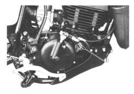
Turn the carburetor pilot air screw inward with a small blade screwdriver until it lightly bottoms, then, back the screw out approximately 1-3/4 turns. This is an approximate setting and may have to be adjusted to suit your geographical area.
