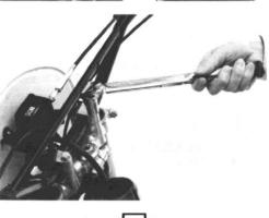
Mount the engine kill switch on the handlebar.
