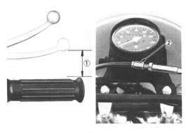
Before adjusting brake pedal travel, adjust brake pedal position with brake pedal adjuster ① until the most suitable position is obtained for quick operation. After adjustment of brake pedal position, adjust brake pedal travel ② with brake cable adjuster ③ to 20  $\sim$  30 mm (0.8  $\sim$  1.2 in).
