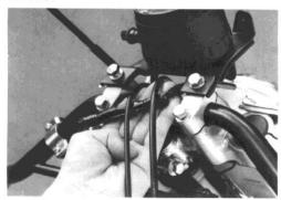
Make sure that the alignment dot is at the mating face of the right clamp.
