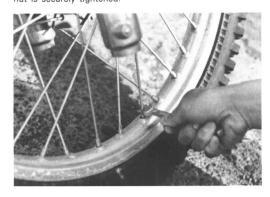
Using an accurate air gauge, check the air pressure of the front and rear tires. The pressure should be front: 0.7  $\sim$  0.9 kg/cm (10  $\sim$  12 psi); Rear: 0.7  $\sim$  0.9 kg/cm (10  $\sim$  12 psi).
