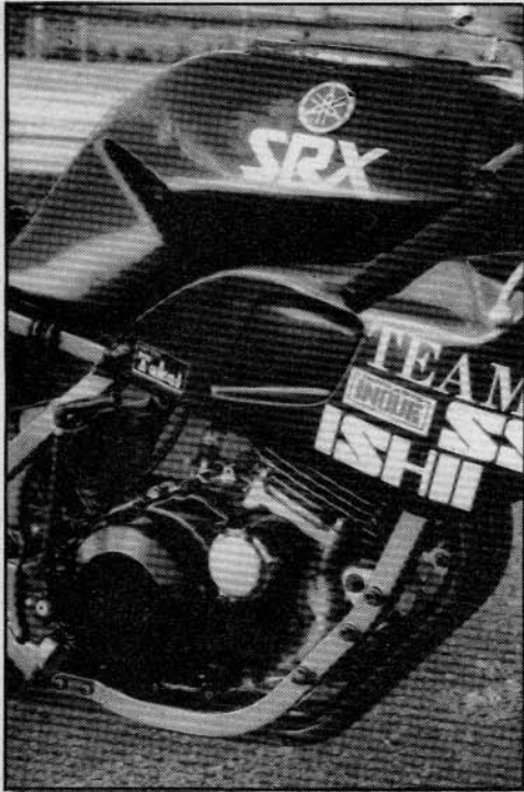
Engine packs lightened and polished conrod and flywheel, high comp piston, big valves, ported head, race cam, bored-out carbs plus a few secret mods — apart from that, it's bog standard!
