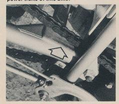
No chain tensioner is used, but nylon "pads" are on top and bottom of swingarm. Top one (see arrow) doesn't wear fast, but the spares kit that comes with the bike includes a couple of the smaller bottom pads, since they will go faster. Simple matter to change them and they're cheap.
