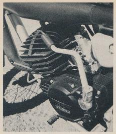
The 125CR's engine is based on the bigger engines in the Husky range. Bottom end is identical, cylinder comes from same mold as the 360cc version. That's why it looks so big. It's a short stroke engine, with a 55x52mm bore/stroke configuration. That's unusual in the 125cc class, but is one of the main reasons for the beautiful power traits of this bike.
