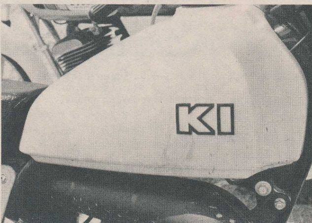
New style plastic gas tank holds 2.2 gallons of pre-mix. Decals aren't much good, however . . . This photo was taken after only two laps of slow practice on the brand new RM400. Tank also has large filler cap, which is very welcome to long-time RM owners.
