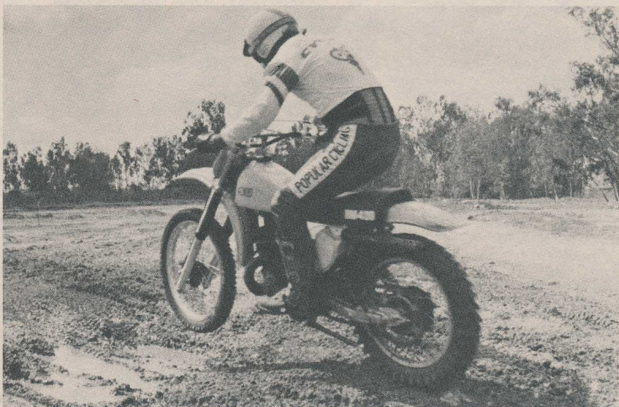
With nearly ten inches of travel on each end, RM400 is state-of-the-art in the suspension department. Also note wide, very effective unbreakable plastic fender, another "trick" detail.
