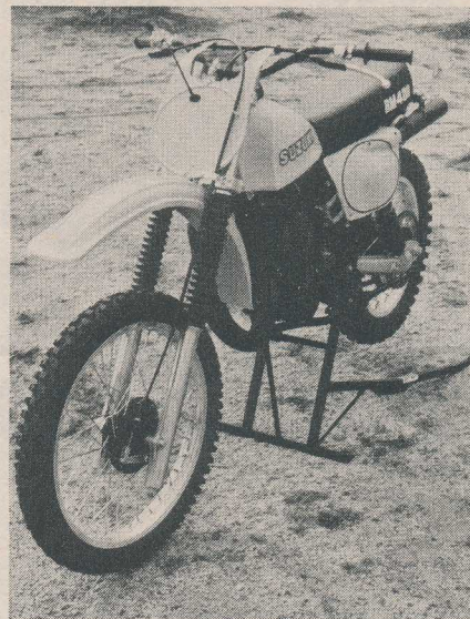
With nearly ten inches of travel on each end, RM400 is state-of-the-art in the suspension department. Also note wide, very effective unbreakable plastic fender, another "trick" detail.
