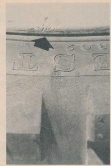
A close-up of this seal shows that it's wearing out, allowing dirt into the bearing which will eventually fall apart. Check the seals every time you pop off the wheels.
