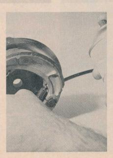
The same sanding technique should be used on the shoes as was done on the drums. Also check the thickness of the shoes with Vernier calipers, and determine, after consulting your owner's manual, if they are too thin and need to be replaced.
