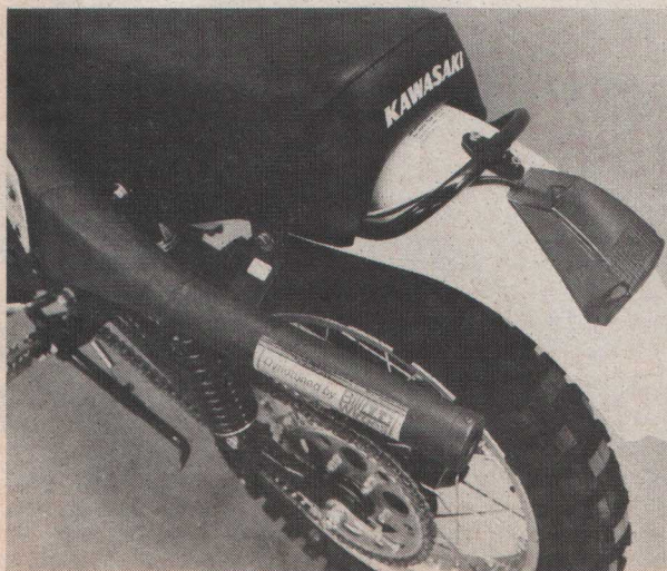
Wirges up-pipe features a rugged rear mounting bracket and a silenced stinger section. All Wirges pipes have internal baffles for additional noise reduction without power loss. The Preston Petty rear fender/taillight combination bolts on easily using the two stock rear mounting bolts and provides lots of extra protection from a muddy spinning rear tire.
