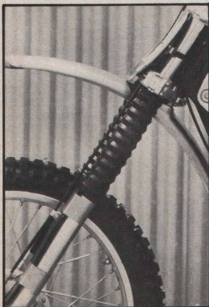
Fork boots protect the tubes; Preston Petty fork garters do it for the sliders.
