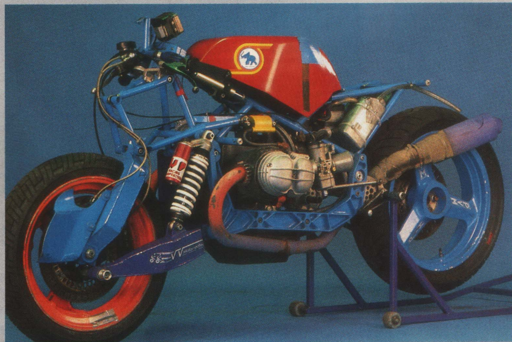
Omit the steering head/fork assembly and road shocks go direct to a super strong cradle.
