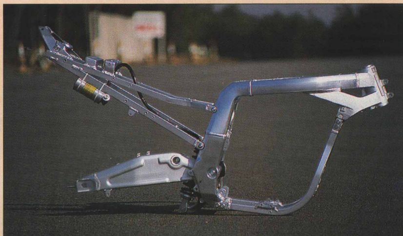
The frame is beefed up (fnarr fnarr) and has an utterly new swing arm. In fact, to cut a long story short, the only things that remains the same as last year's M are the tyres.
