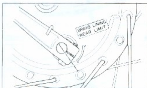
Fig. B The extension line of the index mark is out of the range.
