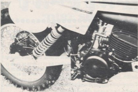
247mm rear end travel matches the front right on.
