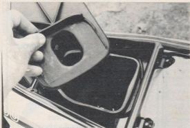
Air cleaner inlet can be enlarged as part of hot-up.
