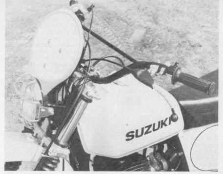
Headlight/number-plate area is tidy, but we wish that Suzuki had used a number-plate of a softer, more flexible material. This one is pretty stiff plastic and could cause substantial injury, in case of a rider going over the bars and trying to take a bite out of the plate. But this is an easy thing for the individual rider to fix on his own.
