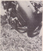
Bash plate is discarded for tube protectors — former is better
