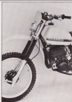
Forks have 38 mm stanchion tubes, damping and spring rates that match the bike perfectly. Front brake is strong and progressive.
