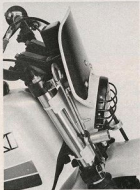
Headlight/number plate combination survived intact. Tools are mounted on triple clamp.
