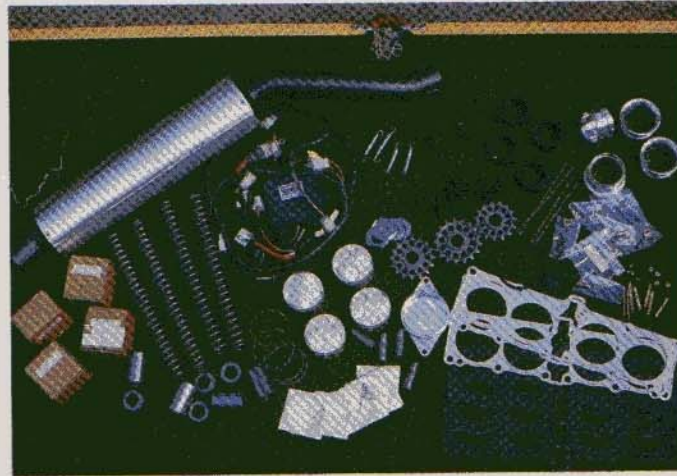
Padgett's also supply the race kit for the OW01 — in essence, all it contains is the noisy tail pipe and the carb kit but you can have refinements like oversize pistons if you really must.
