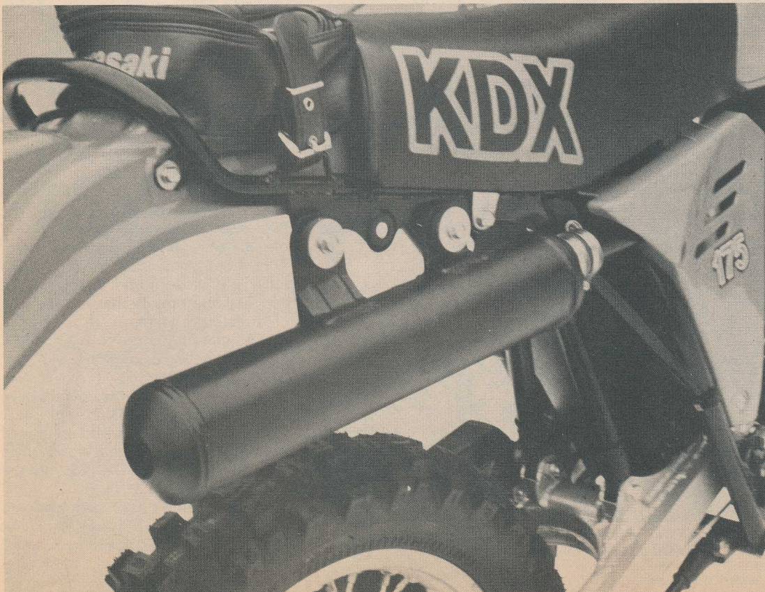
New for 1982 is a larger more effective silencer. The bike can breathe better and turns higher RPM when it's time for fast riding. The mounting position is also balanced and rugged.
