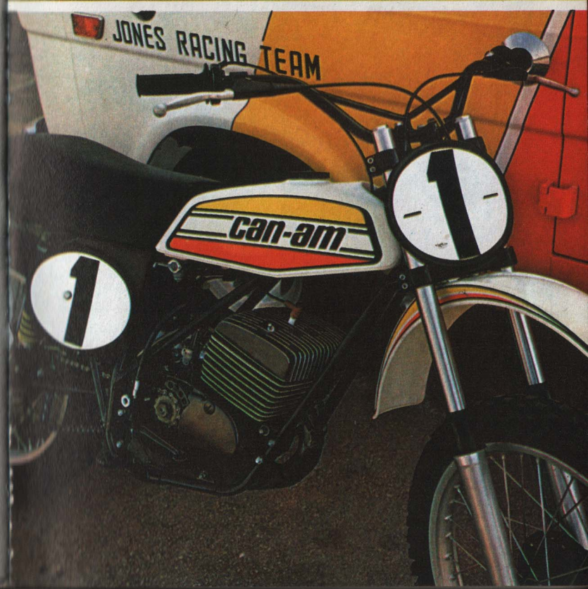
In 1974 Can-Am took a moderate approach in suspension, opting for forward-mount shocks rather than a cantilever system.
