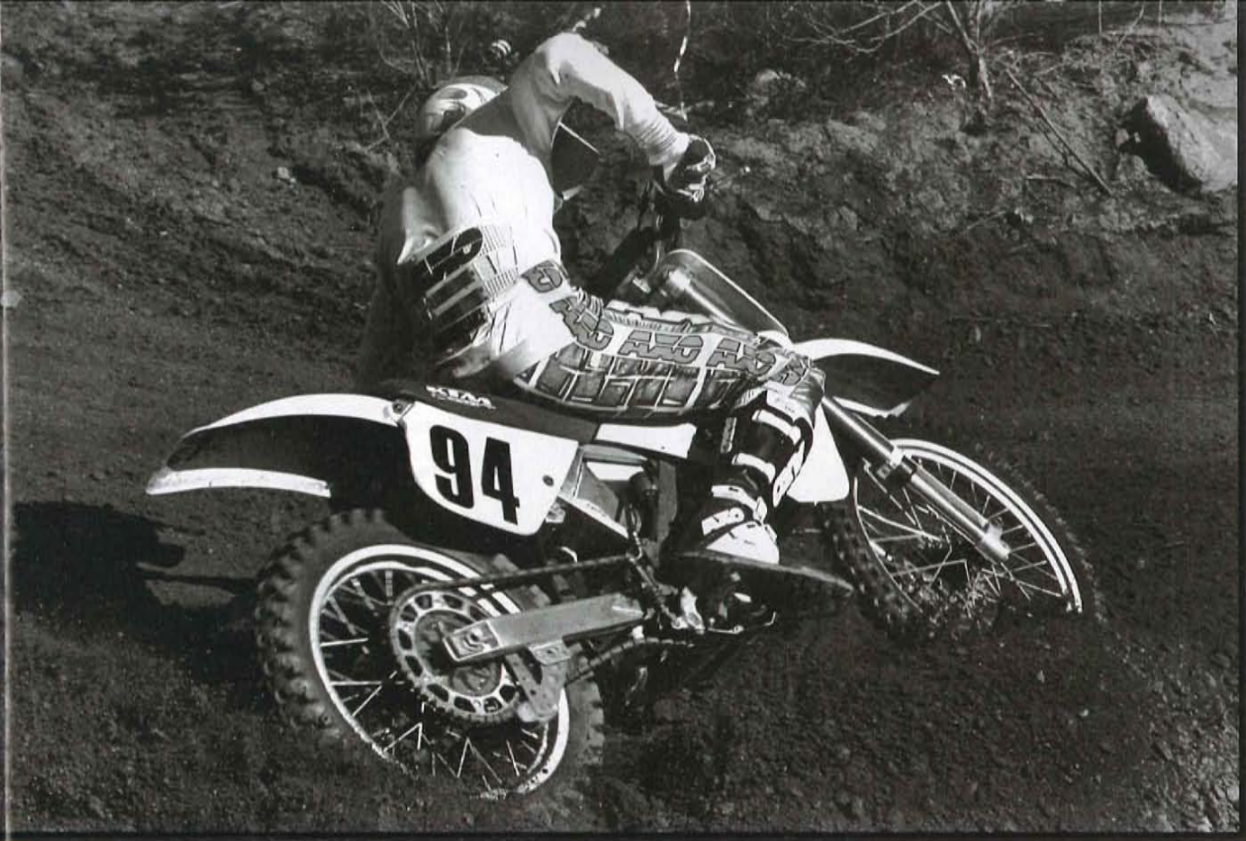
In motion the AMP Research 125 prototype was sleek, slim and trim. Although it was a full-size race bike, the bike was only 10 inches wide at the gas tank/seat juncture. Leitner built the bike as a design exercise, but it could be ridden.
