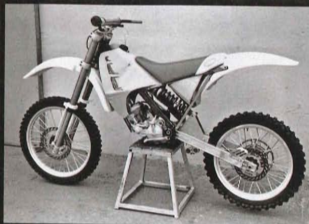
This cardboard mock-up is what the AMP Research 125 was supposed to look like when it was completed. At this stage it lacks most of the finishing touches.
