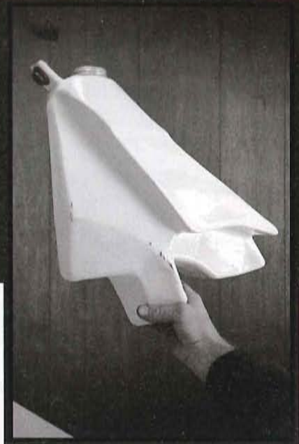
The handmade aluminum gas tank looked small, but held more fuel than most stock 125s of the day. Plus, it sat very low in the frame.
