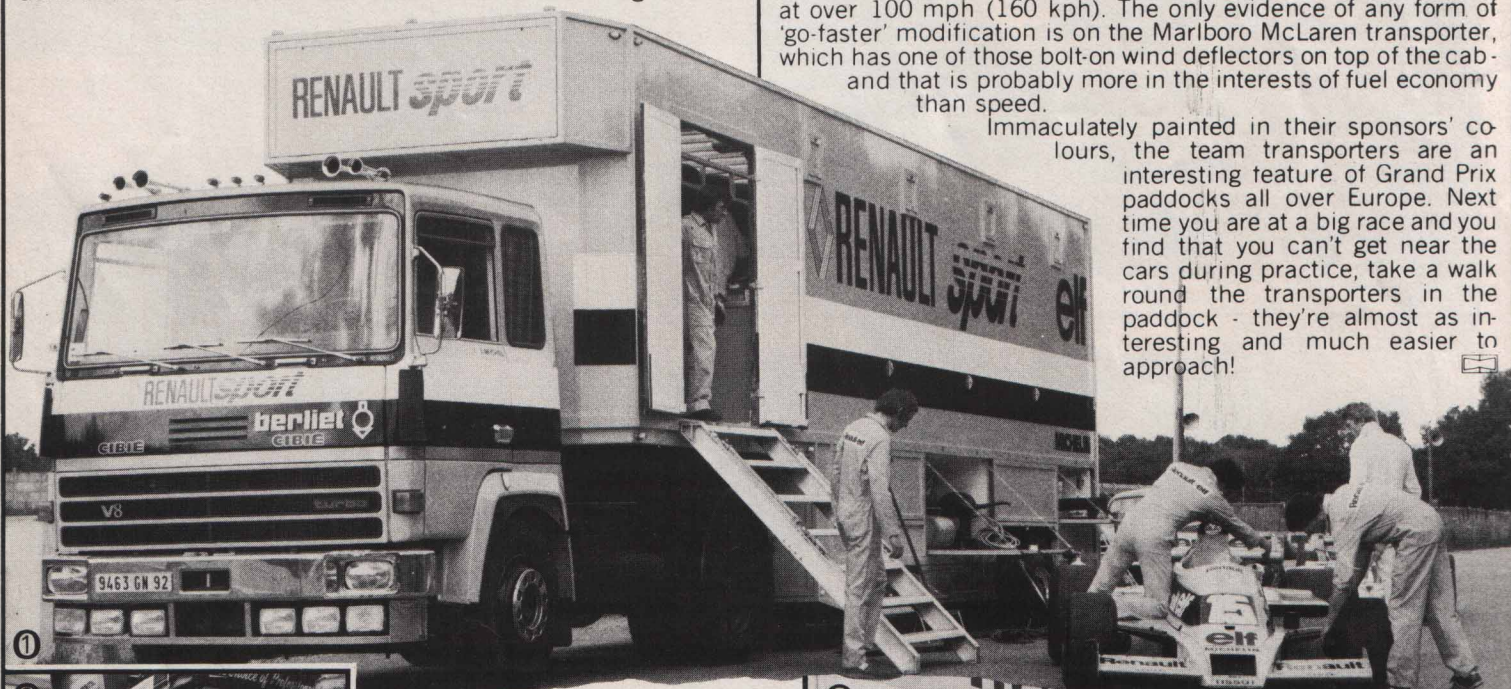
1. The Renault team's transporter is one of the most modern in Formula One and is hauled by a tractor made by the company's Berliet truck subsidiary. Note the storage space built into the sides of the truck. 2. Electric arc welding in the Renault transporter. 3. Working on the cars under the awning fitted to the side of the Renault Formula One team's transporter.
