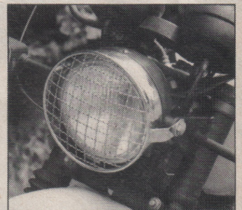
Stone-guarded, rubber-mounted 6in. lamp blew no bulbs
