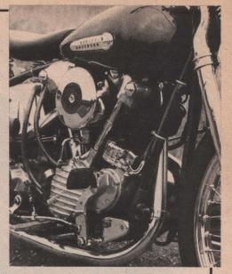
I rubbed my fingers raw cleaning up that frame and then, together with the tank and rear mudguard, I shot it over with a thick coat of Midnight Blue cellulose. The engine came out of hiding and I tore it down to discover two neat score lines down the bore of the rear cylinder. Evidently the gudgeon pin had come adrift at some stage, but fortunately the damage was nothing a rebore couldn't cure.
