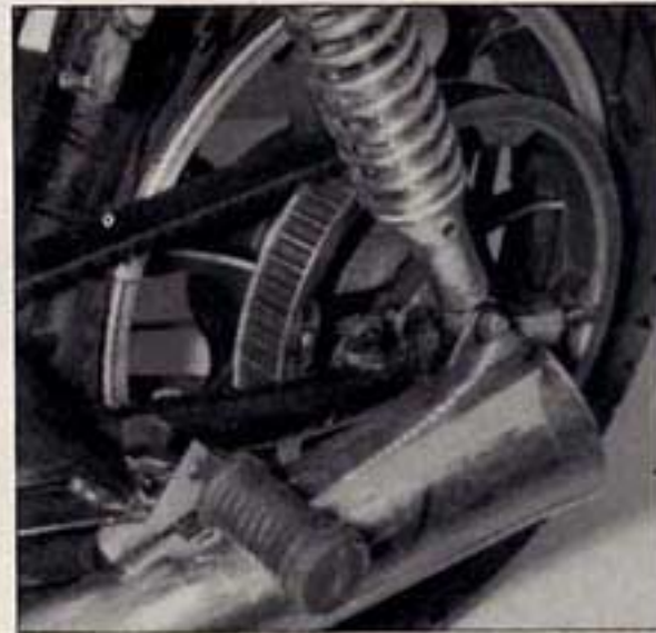
Big, broad rear sprocket is heavy, negating unsprung weight saving of drive belt
