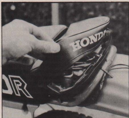
Tool pouch is handy and doesn't get in the way. But it lets in water and gets musty.
